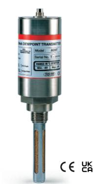
The Alpha Moisture Systems **Model ADHT** is a 4 wire, 4-20 mA, 24V powered dewpoint transmitter. The unit is fully self contained in a robust stainless steel casing with weatherproof protection to IP65, making it ideal for use in heavy industrial environments.
