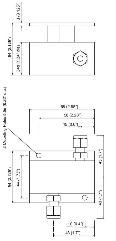
NOTE. The Assembly is shown with 1/4" OD tube fittings. The dimension across the tube fittings will vary for all other size fittings.
