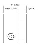
**Note:** The Assembly is shown with 1/4@ OD tube fittings. The dimensions across the tube fittings will vary for all other size fittings.
