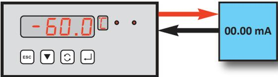
Selecting this range is useful to provide a convenient method of providing a 0-5 Vdc voltage output to the remote equipment when used in conjunction with a suitable 250 Ω resistor.
