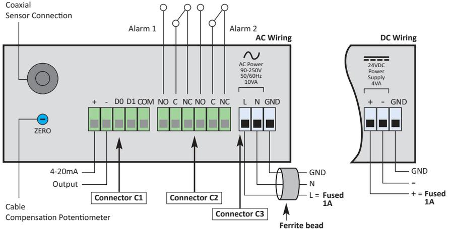
There are three banks of wiring connections points organised into groups named here as C1, C2 and C3.
