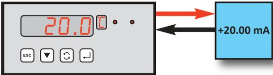
If a sensor is detected as short circuit then the current output will rise to +20.25 mA.
